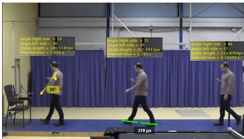
Figure 2: System output for three different moments during monitoring. Example for walking in the scene scenario with ground truth annotations of: step length (middle) and arm-swing angle (left).
