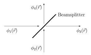
Figure 1: Configuration of incoming and outgoing waves for a beamsplitter.
