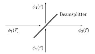
Figure 1: Configuration of incoming and outgoing waves for a beamsplitter.
